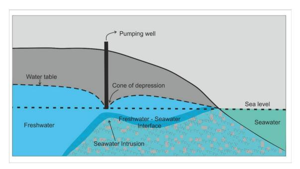
Fig. 1. Schematic diagram of seawater intrusion into the coastal aquifer.
