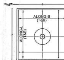
TYP. PLAN OF ISOLATED FOOTING
